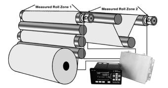
Mode B usually measures two independent tension zones (rolls), each with dead shaft idler roll transducers (4 transducers total). These zones may be two independent points on the same web or any point on two different webs. Mode B analog outputs are roll 1 (transducers 1 & 2) total tension, roll 1 difference, roll two total (transducers 3 & 4), and roll two difference. Mode B also functions with only one, two-transducer tension zone. It is not necessary to use both zones.
